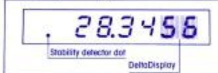
The filling guide (DeltaDisplay) switches on automatically when weighing in substances quickly; the last two digits are blanked out and the display change sequence speeds up. This allows the increase in weight to be followed better. When weighing in slowly towards the target weight, the two digits switch back on.
