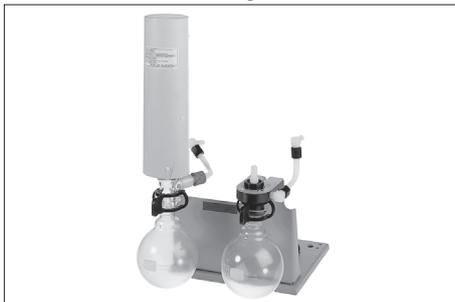
The **exhaust waste vapour condenser** enables an easy and efficient condensation of vapours under atmospheric pressure.
