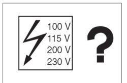
Before switching on the scale, ensure that the line voltage setting matches the local power supply.
