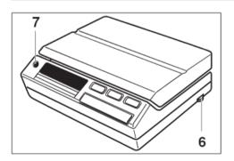
After each relocation of the scale, repeat levelling procedures. For this purpose adjust bubble in level indicator 6 with the two levelling screws 7.
