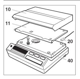
Install platform support 11 with all four pins sitting on rubber grommets 40; then place weighing platform 10 on platform support 11; connect power cable 20.
