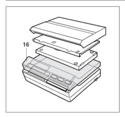
If weighing platform and platform support are already in place, take them off. Then detach protective cover **16** at the adhesive spots and carefully pull off upwards.
