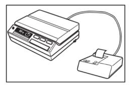
Pressing the PRINT key triggers transfer of a value from the scale to the attached peripheral (printer, e.g. METTLER TOLEDO GA44 or computer).
