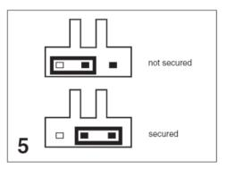
To protect your settings in the configuration file from involuntary changes, position the jumper across **both** contact pins (position **secured**).
