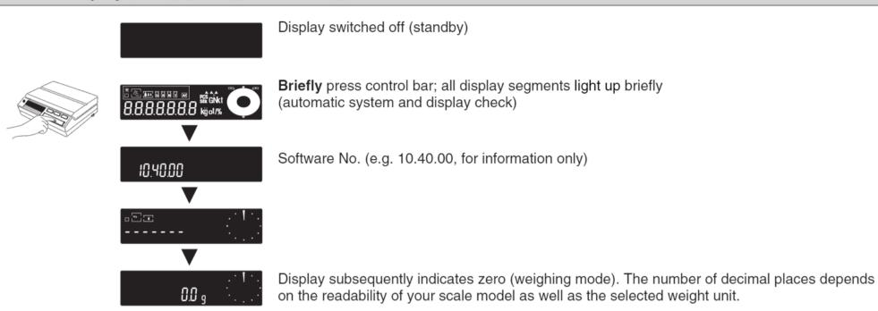
**Note:** Should a power outage occur, the display will indicate -OFF- immediately the power is restored. You should then briefly press the control bar (also consult "What if ...").
