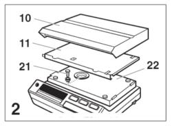
Lift off weighing platform 10 and platform support 11. Undo screw 21. Carefully lift off top housing 22 and place to one side with the display pointing downward.
