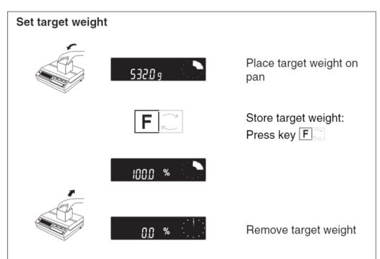
**Note:** If the F-key is pressed again, the weight currently loaded will be stored as a new target weight (100%).
