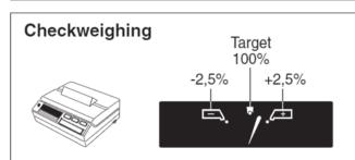
Place sample on platform and check if weight is within tolerance limits.
