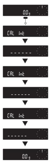
Start calibration with display switched on by pressing and holding the control bar (weighing mode, display zero with empty weighing platform).
