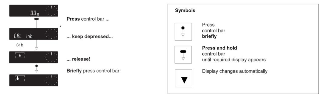
**Note:** If the display automatically returns to zero (weighing mode) **3 seconds** after the control bar was last pressed, simply begin the procedure again.
