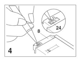
In the aperture of the program cassette **8**, the shorting jumper **24** is now visible. It can be lifted off from the contact pins (e.g. with a small pencil).
