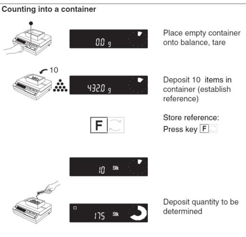
**Note:** If the F-key is pressed again, the weight currently loaded will be stored as a new reference weight for the reference 10 items.
