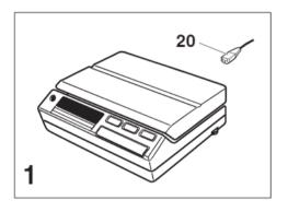
To protect the program cassette from possible interference, it is absolutely essential to first disconnect the line cable **20**.
