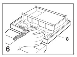
Reinsert the program cassette 8, make sure it is pressed in firmly and fully. Close the scale housing.
