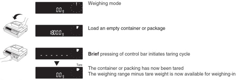
**Note:** The stability detector can be switched off during taring by pressing the control bar twice. It is then possible that the display does not show exactly 0.0 g. The foot or hand switch from the accessories offers the possibility of external taring.
