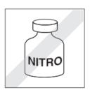
For cleaning the stainless steel platform, a cloth with soap and water is adequate. Never use powerful solvents.
