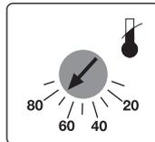
Set the temperature limit using the dial on the rear of the unit. The scale shows approximate temperatures. Set the dial to a value 5-10 °C above the desired working temperature.
