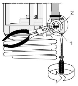
The pump flow is pre-adjusted in the factory and can be modified to suit user requirements.
