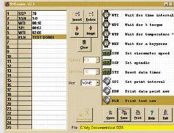
Connect DV-II+Pro to a PC to create a custom test program on your PC and then download test parameters to your viscometer
