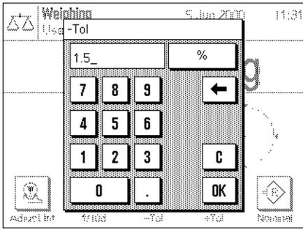
When one or other of the function keys for the minus or plus tolerance is *touched*, the window for entering the corresponding value appears. The input window is the same as for the target value. Here, too, check the unit which is displayed to the right of the tolerance value. You can specify the tolerance as a percentage (%) or as an absolute value in one of the available weighing units.
