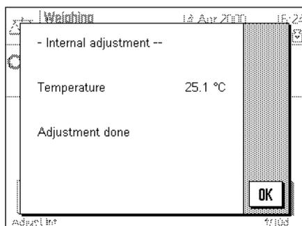
**"Adjustment successfully completed"**. Touch "OK" to return to the application.
