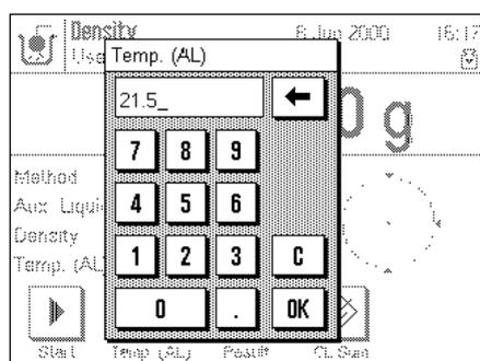
If you use water or ethanol as auxiliary liquid, use the **"Temp. (AL)"** key to enter their temperature (density tables for these two liquids are stored in the balance). The illustration at left shows the corresponding input field.
