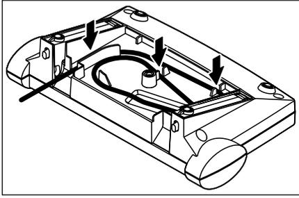
Pull the connecting cable gently out of the tension relievers. Unwind the cable. Replace the cover and fasten it with the knurled screw.
