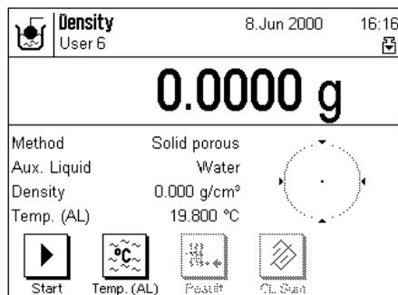
In the application-specific settings select the method **"Solid porous"** (Section 8.3.2) and specify the desired auxiliary liquid (Section 8.3.3).
