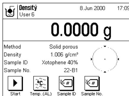
You can also activate the two information fields "Sample ID" and "Sample No." (section 8.3.5) so that the texts and numbers you have entered are also shown in the display.
