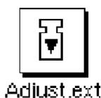
By touching this function key, you start adjustment (calibration) of the balance using an external calibration weight. **Note:** Depending on country-specific regulations, this function may not be available on certified balances.
