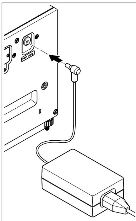
Your balance is delivered complete with an AC adapter and a country-specific power supply cable. The AC adapter is suitable for all power supply voltages in the range: 100 – 250 VAC, -10/+15%, 50 – 60 Hz.
