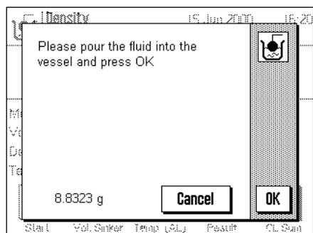
After a short pause you will be prompted to pour the liquid whose density is to be determined into a container. If you are working with the below-the-balance hanger, place the container with the the liquid in it under the hanger. If you are working with the optional density kit, follow the instructions delivered with the kit. In either case, ensure that the sinker is immersed at least 1 cm in the liquid and that there are no air bubbles in the container.
