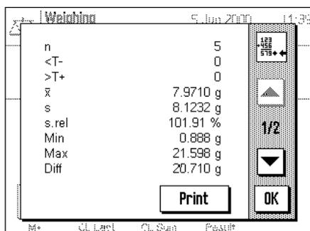
After you have touched the "Result" function key, the results of the weighing series appear in the display. You can use the arrow keys to page backward and forward between the different screen pages.
