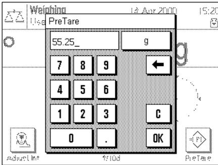
Key the desired tare value in. Check the weighing unit: this is displayed to the right of the tare value. If you touch the weighing unit, the units available for selection are displayed. **Note:** The units are not converted automatically, i.e. if you input a value in a particular unit, this value remains, even if you change the weighing unit.
