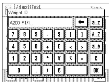
Here you can assign a designation to the adjustment weight used (max. 20 characters). This makes identifying the adjustment weight easier. The weight identification is then printed on the adjustment report. The same alphanumeric input window appears as for the certificate designation.
