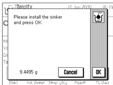
Touch the "Start" function key to start the density determination. After a short pause, you will be prompted to mount the sinker (for weighing in air).
