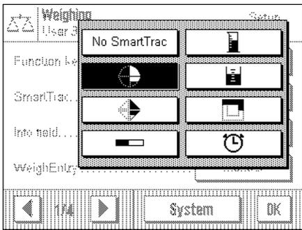
You can choose between various different display modes for "SmartTrac", or turn it off. Also, instead of "SmartTrac", you can display a stopwatch.
