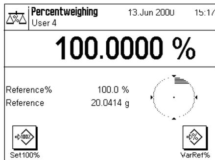
Place the reference weight on the weighing pan.
