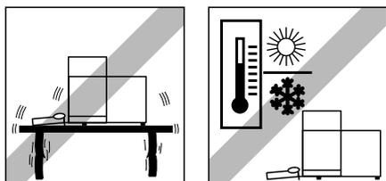
Choose a position which is stable, free from vibration, and as nearly horizontal as possible. The supporting surface must be able to bear the weight of the fully loaded balance safely. A stone table is recommended for MX/UMX balances.
