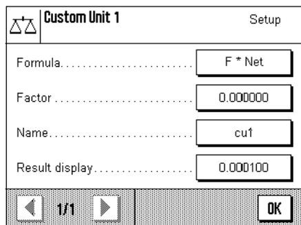
You can use a custom weighing unit to perform calculations based directly on the weighing result as soon as it is obtained (e.g. for surface areas or volumes). The custom weighing units are available in all menus and input fields in which you select weighing units.
