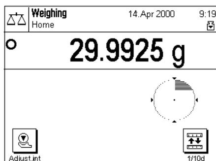
As soon as the stability detector symbol (the small ring to the left of the weight display) goes out, the display is stable and you can read the weighing result. In the illustration at the side, the stability detector symbol is still visible, and the weighing result is therefore not yet stable.
