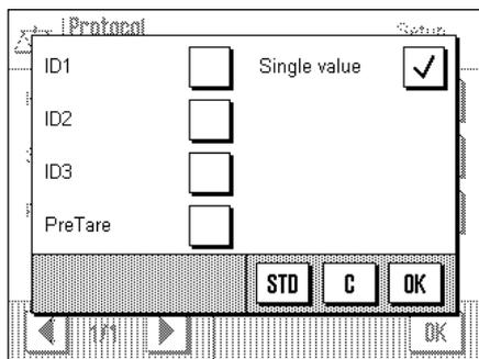
In this submenu you specify the information to be printed on the record for each individual weighing result.
