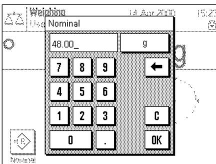
When the function key is touched, the window for entering the target weight appears.
