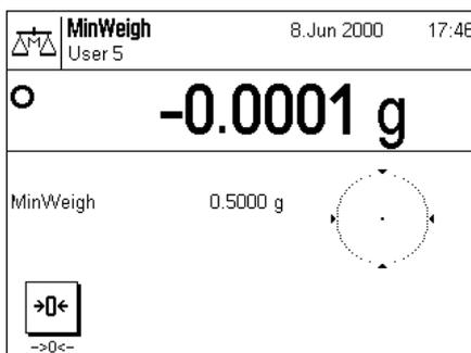
When you have selected the application, the display shown at left appears. The special minimum weighing function key and information field have been activated at the factory. You can change these settings to suit your needs according to the description in the sections that follow below. The value shown for minimum weighing (0.5 g in the example shown at left) is calculated from the respective tare weight and the programmed values and cannot be changed.
