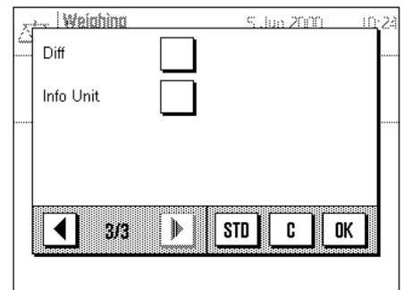
In this menu you specify which information fields should be displayed in the application. You can call up the menu for the information fields directly from the application by touching the corresponding zone of the display (Section 4.2).
