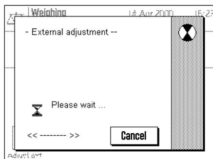
If the automatic door function is active, the glass draft shield closes automatically after you have placed the weight on the pan; otherwise, you must close it manually by touching the «↕» key. While adjustment is taking place, the window shown on the left is opened. You can terminate the adjustment process at any time by touching the "Cancel" key.
