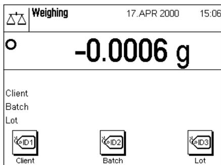
The example on the left shows the balance display after the ID function keys, and the ID information fields, have been activated.
