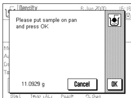
Touch the **"Start"** key to start the density determination. After a short pause you will be prompted to place the solid on the weighing pan for the first weighing in air.
