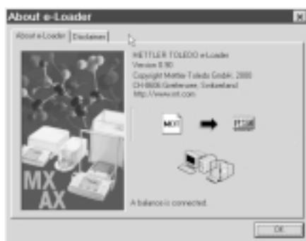
Use the "Help" menu to check that the communication with the balance is functioning (in the example at left, the e-Loader is confirming that a balance is connected).
