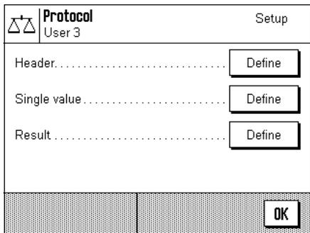
To make it clearer, this extensive menu is divided into 3 submenus in which you can specify the options for the title of the record, recording the individual values, and the weighing result.
