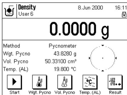
In the application-specific settings select the method "pycnometer" (Section 8.3.2).
