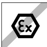
The balance may only be used in enclosed interior rooms. It is not permitted to use the balance in hazardous environments.
