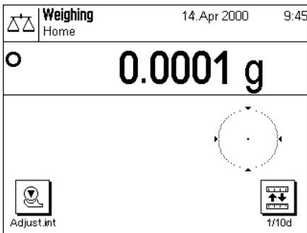
**Switch on the balance:** Switch on the balance by briefly pressing the «On/Off» key. After the balance has been switched on, it is in the "Home" profile of the "Weighing" application. **Important:** While you are working, you can return to the "Home" profile at any time by touching the «⏪» key.
