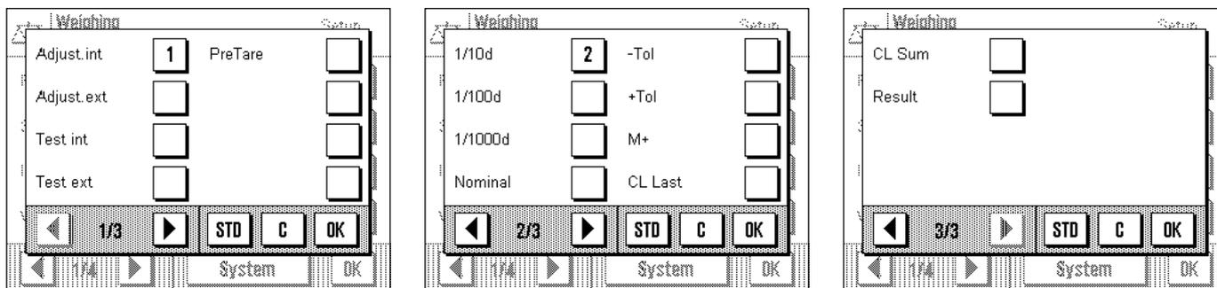
In this menu you specify which function keys should be available in the application. You can call up the menu for the function keys directly from the application by touching the corresponding zone in the display (Section 4.2).
