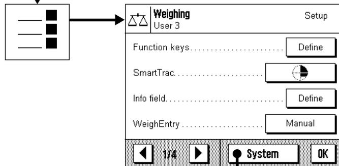
Settings for the selected application (the example shows "Weighing") are stored in the active user profile (in the example, "User 3").
