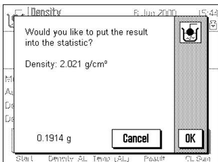
The balance now determines the density of the solid, and you will then be asked whether you wish to accept the result of the density determination into the statistics.
