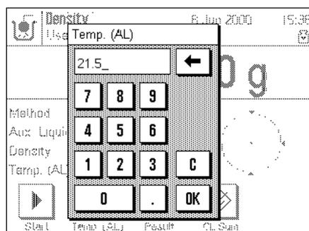
If you use water or ethanol as auxiliary liquid, enter the temperature using the function key "**Temp. (AL)**" (density tables for these two liquids are stored in the balance). The illustration at left shows the input field to be used.
