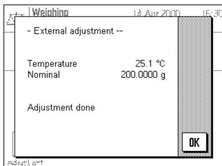
The balance confirms successful completion of the adjustment. Touch "OK" to return to the application.
