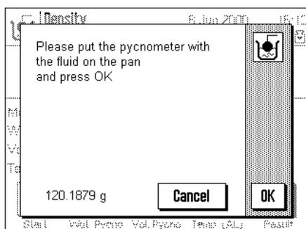
Touch the "Start" function key to start the density determination. After a short pause you will be prompted to place the filled pycnometer on the weighing pan.
