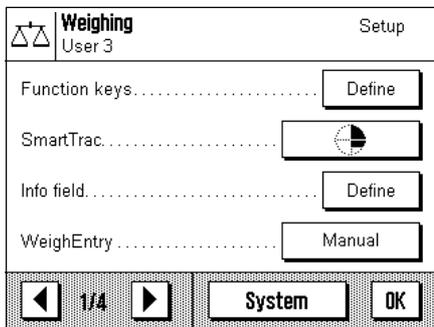
**"Function keys":** Here you can specify which function keys should appear at the bottom edge of the display. These keys allow direct access to certain functions (Section 6.2.2).
