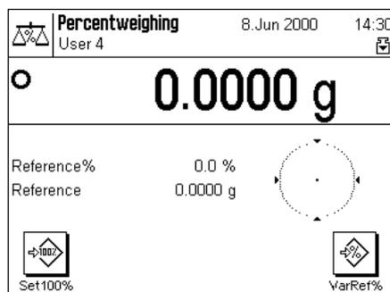
After you have selected the application, the display shown at the left appears. Before leaving the factory, the special function keys and information fields for percent weighing have been activated. You can adapt these settings to your needs according to the descriptions in the sections that follow.
