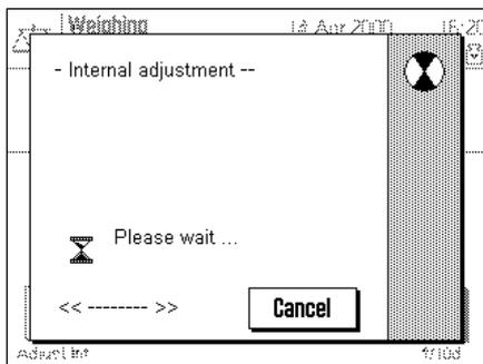
You can hear the motor placing the internal weight on the weighing pan and then removing it again. While adjustment is taking place, the window shown on the left is opened. You can terminate the adjustment process at any time by touching the "Cancel" key.
