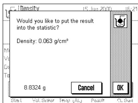
The balance now determines the density of the liquid, and you will then be asked whether you wish to accept the result of the density determination into the statistics.
