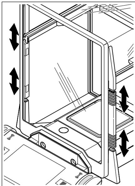
The position of the coupling elements determines which parts (left-hand, right-hand, and upper door) of the glass draft shield can be opened.
