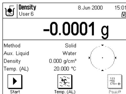
When the application is selected for the first time, the display shown at left appears. Before leaving the factory, special function keys and information fields for density determination have been activated. The balance is set for performing density determination of solids using water as auxiliary liquid. You can change these settings to meet your needs as described in the sections following below.
