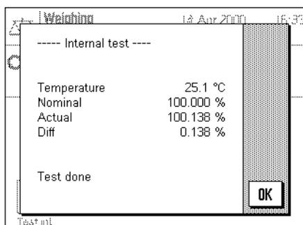
The successful conclusion of the checking procedure is confirmed with the window shown on the left. If a printer is connected to the balance, a record of the check is automatically printed out according to the system settings you selected for adjustment and test (Section 5.3). You will find an example of a record in Section 6.4.6.
