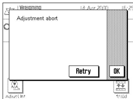
**"An error has occurred while adjusting and the adjustment has been terminated."** This message also appears if you terminate the adjustment yourself. You can repeat the adjustment process or return to the application by touching "OK".
