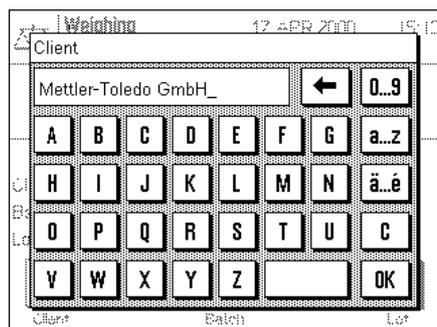
In the application, when you process a job for a client, and when weighing is complete, touch the "ID1" ("Client") function key and a field appears to input the client (see illustration at left). Enter the name, and confirm your input with "OK".
