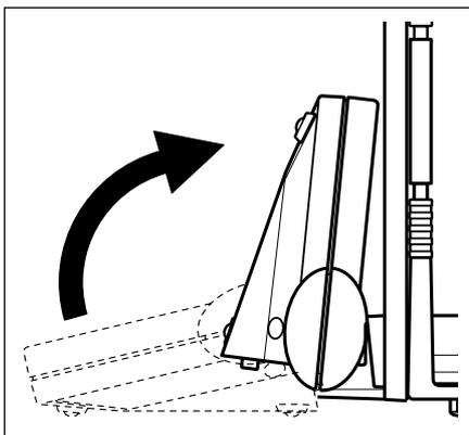
Unscrew the knurled screw underneath the terminal and remove the cover.
