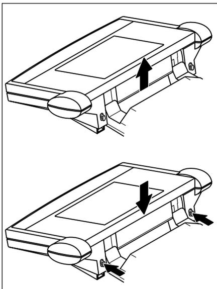
If you wish to have a flatter reading angle, press the two stop buttons on the back of the terminal and press the terminal downward. Release the two stop buttons and the terminal will then click into the desired position.
