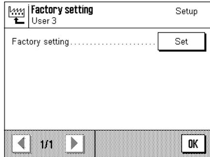
Here you can reset all the settings to the factory settings. **Important: Resetting affects all the settings (application-dependent settings and system settings) for the active user profile!**
