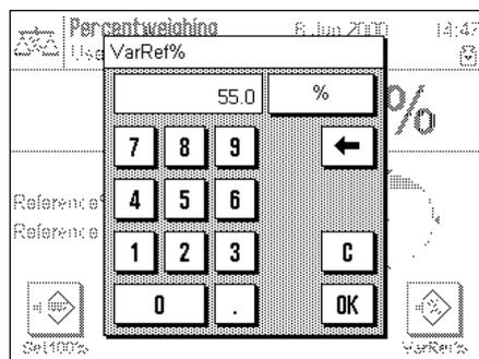
If you wish to assign a **variable reference** to the weight on the pan, touch the "VarRef%" key instead. An input field appears in which you can enter the percentage value (e.g. 55%) to which the weight on the pan should correspond.
