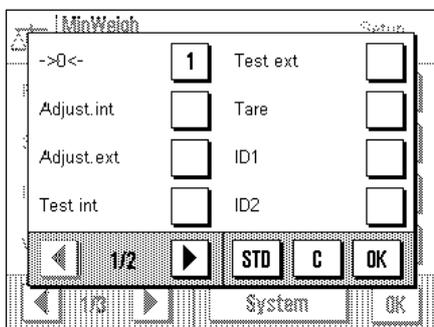
**"->0<-":** You can use this function key to reset the display value to zero. Since the minimum weighing value is significantly affected by the tare value, a difference has to be made between taring and zeroing (resetting the display to zero). Use this function key to reset the display to zero, and for taring use the «→0/T←» key on the terminal.
