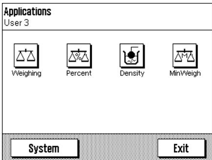
**Select application:** If you do not wish to work with the weighing application, use the «☐☐☐» key to select the applications menu. (Alternatively, you can touch the corresponding zone in the top left-hand corner of the display). Touch the symbol for the desired application and the software will load the application.
