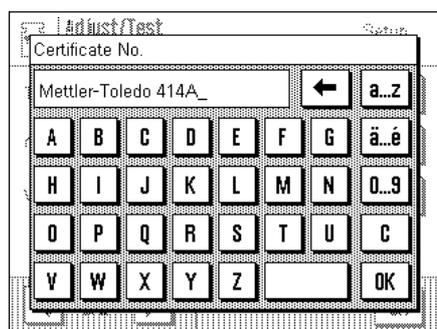
Adjustment weights are generally delivered with a certificate. You can enter the designation and/or number of the certificate delivered with the weight here (max. 20 characters). This makes it possible to unambiguously link the adjustment weight used to a specific certificate. The certificate designation is then printed out on the adjustment record. The input window allows input of alphanumeric characters.
