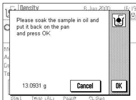
After a short pause you will be prompted to immerse the solid in the oil bath and then to replace it on the weighing pan (or hanger) for the second weighing in air.
