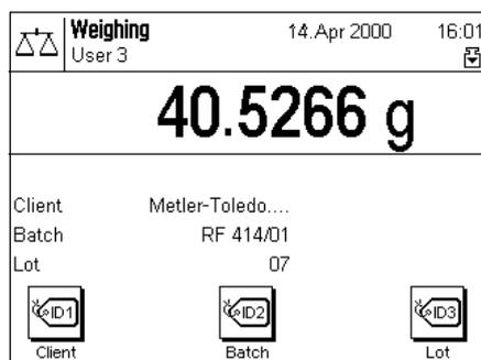
When you have completed all the inputs, you can again check the identifications you have selected by means of the information fields in the display.
