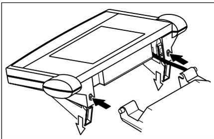
Press the two stop buttons on the back of the terminal and pull the terminal further upward. By doing this you release the two feet of the terminal from their mountings. Place the terminal in the desired location. Press the two stop buttons and lower the feet back into the terminal.
