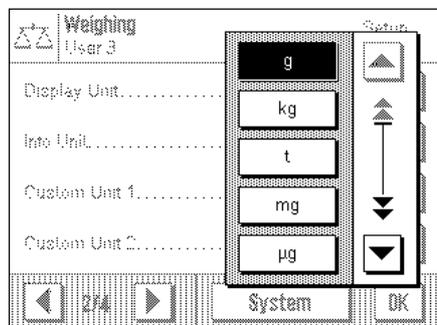
The same selection of units is available for both the "Display Unit" and the "Info Unit". When the "Display Unit" is changed, the current weighing result, the saved weighing results (sum), and the statistical values are displayed in the new unit. On the other hand, the values for tare preset, target weight, and tolerances are still displayed in the unit which was selected at the time these values were defined.
