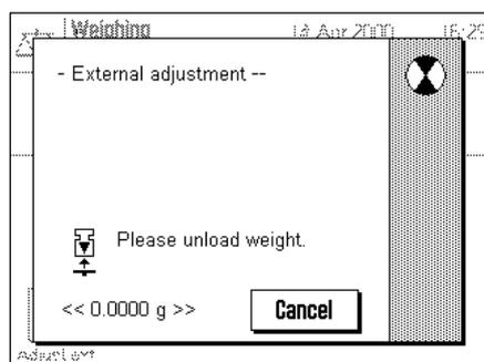
When the adjustment process is complete, you will be prompted to unload the weight. Remove the weight from the weighing pan.
