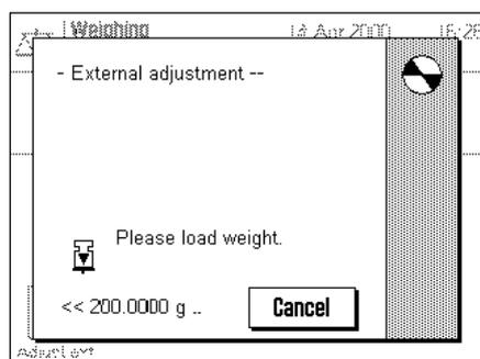
You are prompted to load the adjustment weight onto the pan. The weight needed for adjustment is shown at the bottom edge of the window. If the automatic door function is active (Section 5.7), the glass draft shield opens automatically for you to place the weight on the pan.
