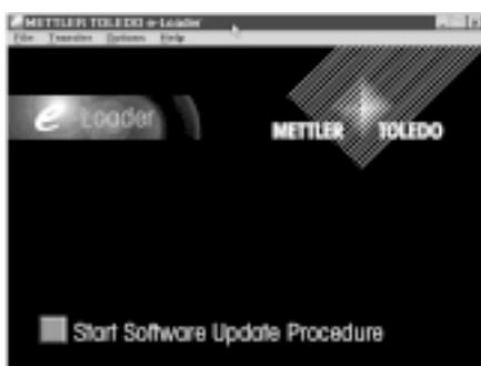
When the installation is complete, the e-Loader starts automatically. The illustration at left shows the startup screen of the e-Loader.
