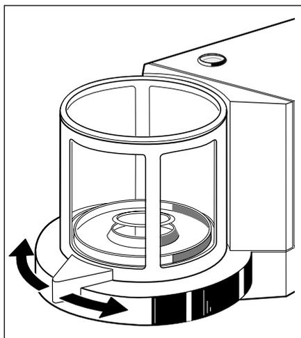
The glass draft shield can be opened and closed either by means of the «↕» key, the "SmartSens" sensors, or by turning the door handle by hand. The door keys and "SmartSens" sensors will be described in detail later in these operating instructions.
