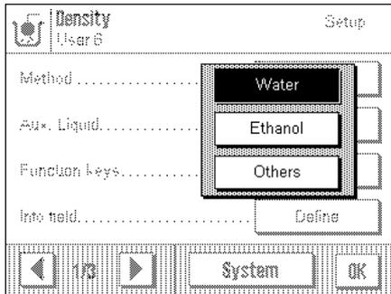
**"Water"**: Distilled water is used as the auxiliary liquid. The density of distilled water at various different temperatures is stored in the balance (density table from 10 °C to 30 °C) so it need not be known.
