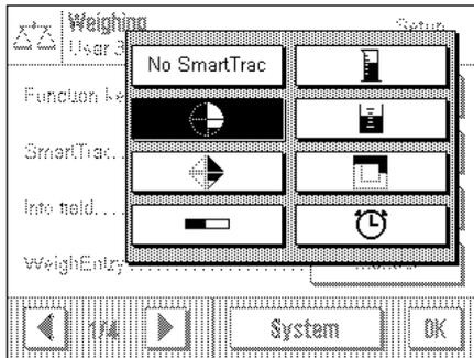
In this menu you can select the display mode for "SmartTrac" or switch it off. Instead of "SmartTrac", you can also display a stopwatch.
