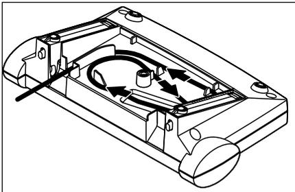
To fasten the terminal onto the balance or control unit again, carry out the procedure in the reverse order. Please refer to the illustration on the left: it shows how to place the cable correctly in the terminal housing.
