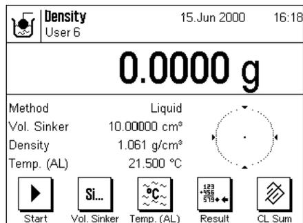
In the application-specific settings, for the method select "Liquid" (Section 8.3.2).
