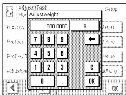
If you work with an external adjustment weight, you can define its weight and unit here. (**Note:** Depending on country-specific regulations, this function may not be available for certified balances). An input window appears which looks like a pocket calculator and can be used like one. Enter the weight of the external adjustment weight. Check the weighing unit: it is shown to the right of the weight. If you touch the weighing unit, the selection of available units appears.
