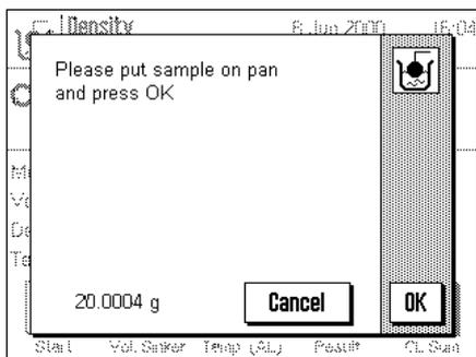
Touch the "**Start**" function key to start the density determination. After a short pause you will be prompted to place the sample on the weighing pan (without the gamma sphere).
