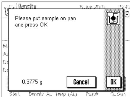
Touch the "**Start**" function key to start the density determination. After a short pause you will be prompted to place the solid on the weighing pan (weighing in air).
