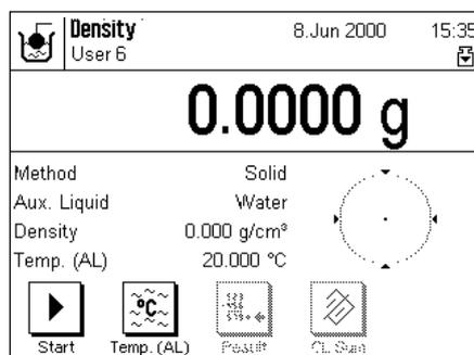
In the application-specific settings select "**Solid**" as the method (Section 8.3.2) and specify the desired auxiliary liquid (Section 8.3.3).
