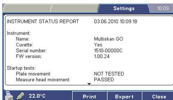
The status report provides current information on the instrument status, including the instrument model and serial number, firmware version, current temperature and other parameters.
