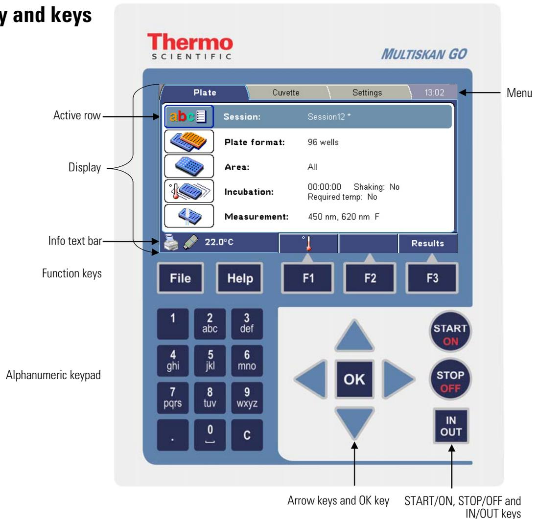
**Figure 5–14.** Keypad and display of the Multiskan GO
