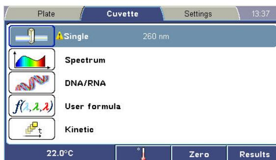
Cuvette sessions or measurement results cannot be stored in the instrument’s memory. You should export or print measurement results if you wish to use them later. The instrument memorizes the most recent measurement parameters and results for each predefined session type.
