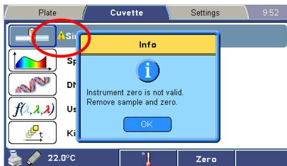
When Zero is pressed, the instrument measures the current absorbance level and sets it to 0.000 Abs.
