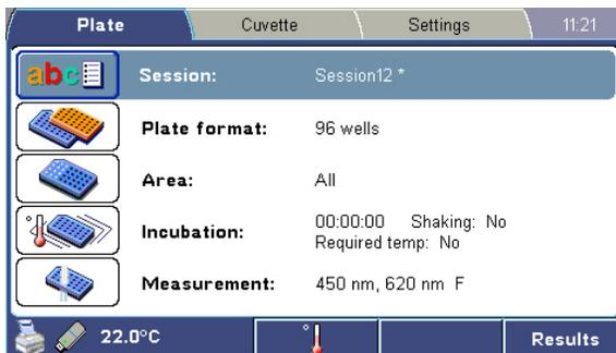
The asterisk (\*) by the session name indicates unsaved results. These are retained until new results are generated. To store results for later use, you should save them in the instrument's memory, export them to a connected USB memory device or print them on a connected USB printer.
