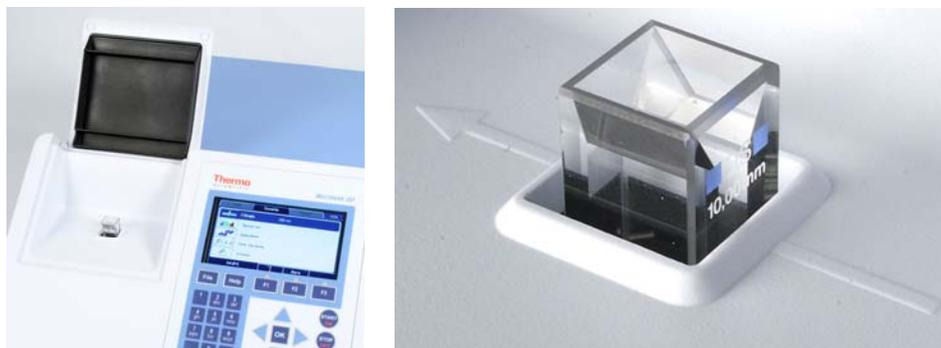
**Figure 4-13.** Multiskan GO cuvette port
