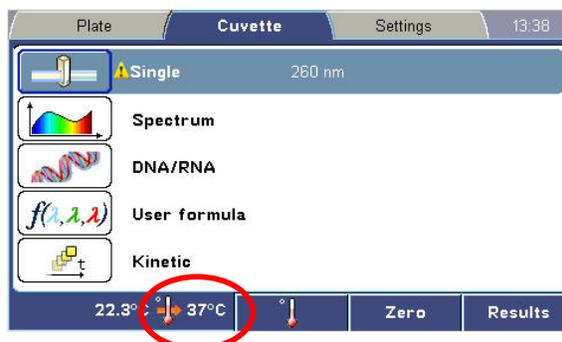
You can toggle the instrument incubator on and off with the F1 key. When you turn off the heating, the heating icon blinks for a few seconds.
