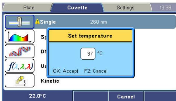
The temperature setting range is 10–45°C with a resolution of 1°C. When the heating is on and the temperature set, the target temperature is displayed on the info text bar (see below).
