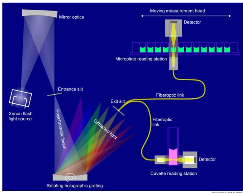
Figure 2–6. Multiskan GO with cuvette optical system
