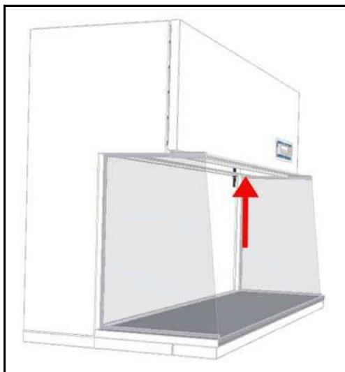
Figure 12 Position of the FL-tube
