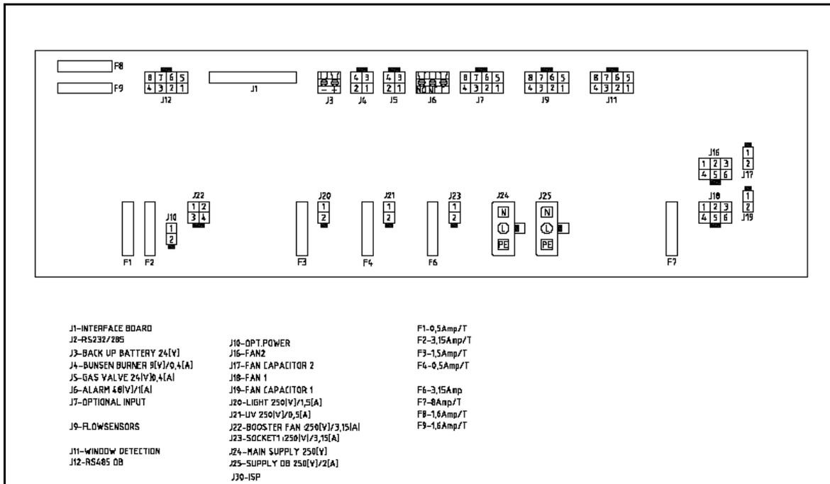
Figure 15 Control board E010001 rev F
