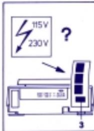
Before starting to use the balance, make sure it is set to the right supply voltage.
