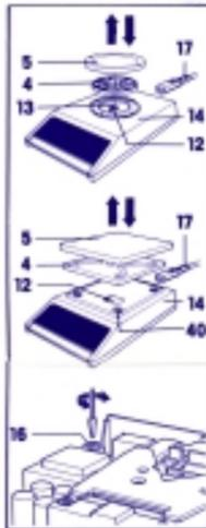
First make sure that the mains cable 17 is disconnected. With the mains cable plugged in, the inside of the balance is under voltage, even when the display is blank! Take off pan 5 and pan support 4, remove screw 12, carefully raise upper housing 14 and alter voltage selector 16 with a screwdriver.
