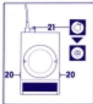
If the balance is moved to a new place, it must be re-leveled each time. To do this, adjust the position of the bubble in the level indicator 21 by means of the screw feet 20.
