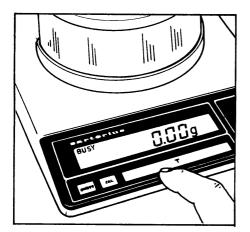
If you wish to use a Container to weigh or if the weight display does not indicate 0.00 g (or the equivalent with the weight unit of your choice), press the tare control to zero the display.
