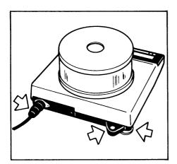
At the point of use, level the balance using the leveling feet (7) so that the air bubble is centered within the circle of the level indicator (14) (for modeis L 220 S, L 420 P and L 420 S only).
