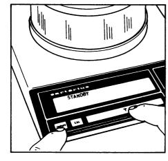
After you have accessed the menu of the operating program, the display will show a continuous sequence of numbers from 0-5 for the "page" or first digit of the code, in addition to the Status code letter "L" or "C."
