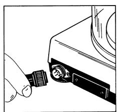
Plug the AC adapter cord into the power receptacle of the balance. Secure the connection by tightening the knurled collar. Now plug the AC adapter into a wall outlet.
