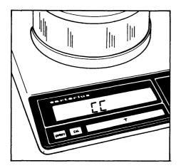
After a few seconds, the display will indicate "CC" followed by 0.000 g. An acoustic Signal indicates the end of the calibration procedure.
