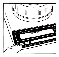
Press the ON/OFF key (11) to switch the balance on or off. You can also turn on the balance with the tare control (9).
