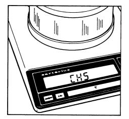
After the power is tumed on, a test of all essential functions is run automatically.
