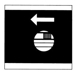
To do so, remove the protective cap located on the front right of your balance and slide the menu access switch (8) in the direction of the arrow.
