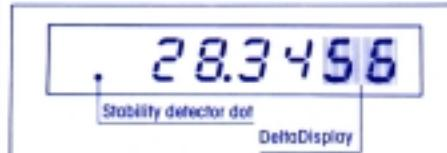
The filling guide (DeltaDisplay) switches on automatically when weighing in substances quickly; the last two digits are blanked out and the display change sequence speeds up. This allows the increase in weight to be followed better. When weighing in slowly towards the target weight, the two digits switch back on.
